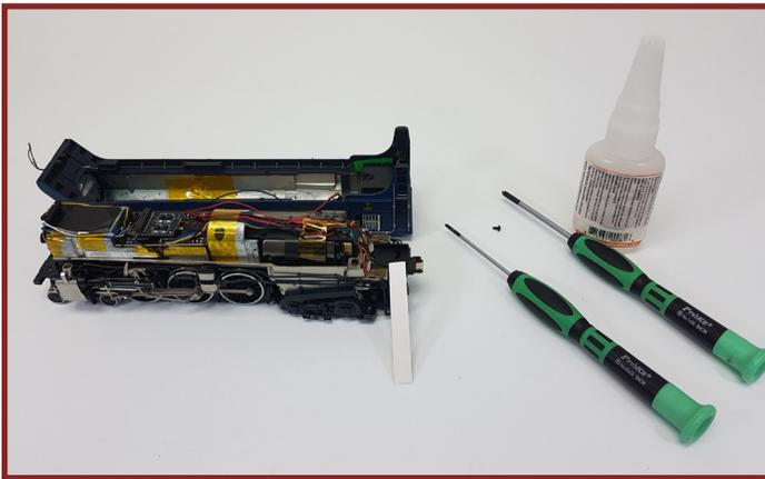
The intermittent chuff or total loss of chuff is due to the motor top cover shifting from its locked position, owing to excessive play in the locking tabs. The fix is fairly easy and can be carried out with tools and other items you may already have available. You can also request a **Rapido Chuff Repair Kit** from us and we will mail you one at no charge.
